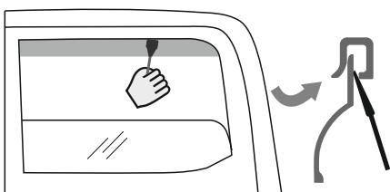
9. To ensure better installation of the deflector and better adhesion between the tape and the surface of the rubber seal, it is strongly recommended that you use the plastic blade, moving it slowly between the window's inner rubber seal and the deflector.
