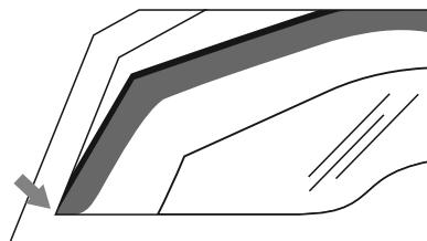
3. Place the front part of the deflector onto the lower frame of the window as shown in the picture.
