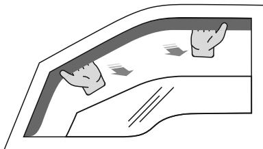
7. Immediately after installing the deflector, adjust its position by carefully pulling it outwards.
