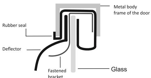
4. The picture demonstrates how to position the fastening bracket.
