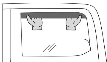
8. Immediately after installing the deflector, adjust its position by carefully pulling it outwards.
